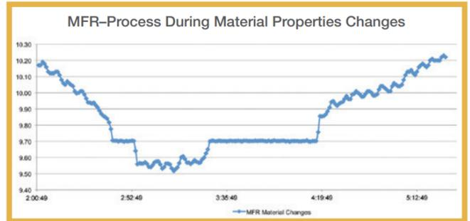
The above graph shows process readings taken by the ViscoSensor during relatively consistent material processing. With consistent Melt Flow Ratio (MFR), one knows the material is homogenous as well as molecular weight concluding that polymer chain branching is staying constant.
