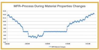
The above graph shows process readings taken by the ViscoSensor during relatively consistent material processing. With consistent Melt Flow Ratio (MFR), one knows the material is homogenous as well as molecular weight concluding that polymer chain branching is staying constant.
