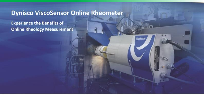
A capillary viscometer forces material through a small diameter capillary die creating a pressure drop across the die. By controlling the material's shear rate through the die or shear stress across the die, apparent viscosity or melt flow index is obtained. The ViscoSensor uses differential pressure across the capillary die for either a control point for melt flow index measurement or as a measurement point for apparent viscosity calculations.
