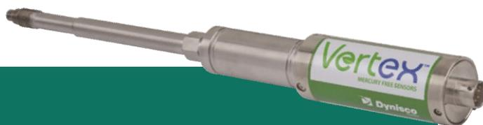
CMR IV has been updated to include Dynisco's advanced-performance Vertex, mercury free sensors offering longer life, faster response, and mercury free operation. By updating the Rheologic Sensing Unit (RSU) with Vertex the processor will have longer life, and higher accuracy (especially at low pressure requirements). The Vertex unit is fitted to the CMR IV with a M18 to 1/2-20 adapter which enables us provide a retrofit kit to existing units in the field.
