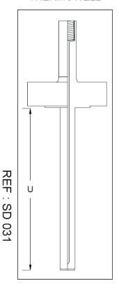
TAPERED STEM RJT RING JOINT TYPE FLANGED THERMOWELL
