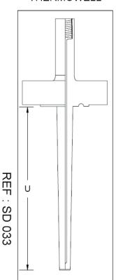
WELD IN CONNECTION BAR STOCK THERMOWELL
