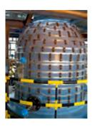
Continuous Thermocouples generate a measurable voltage like normal thermocouples, however, the measuring junction in a Continuous Thermocouple is not formed by directly joining the two wires. More remarkably, the measuring junction is not fixed but, when subjected to an increase in temperature, becomes concentrated at the hottest point anywhere along the sensor's entire length. This is due to the large fall in resistance in the insulating material at the heated area.
